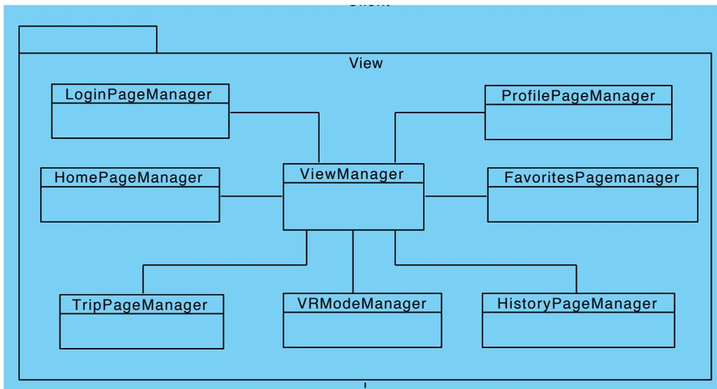
Figure 6 - View Subsystem in Client
