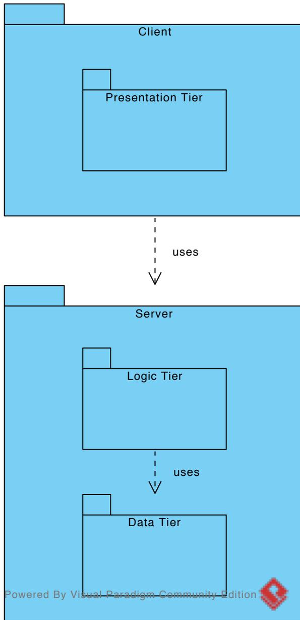
Figure 1 - Subsystem Decomposition
