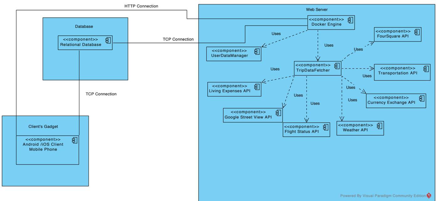
Figure 3 - Component Diagram
