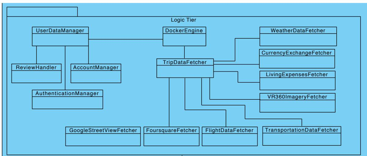
Figure 8 - Logic Tier Subsystem of Server
